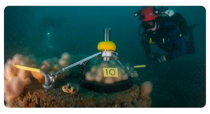
Image Credit: Joost van Uffelen. Incubation of the fouling community using an incubation chamber.
